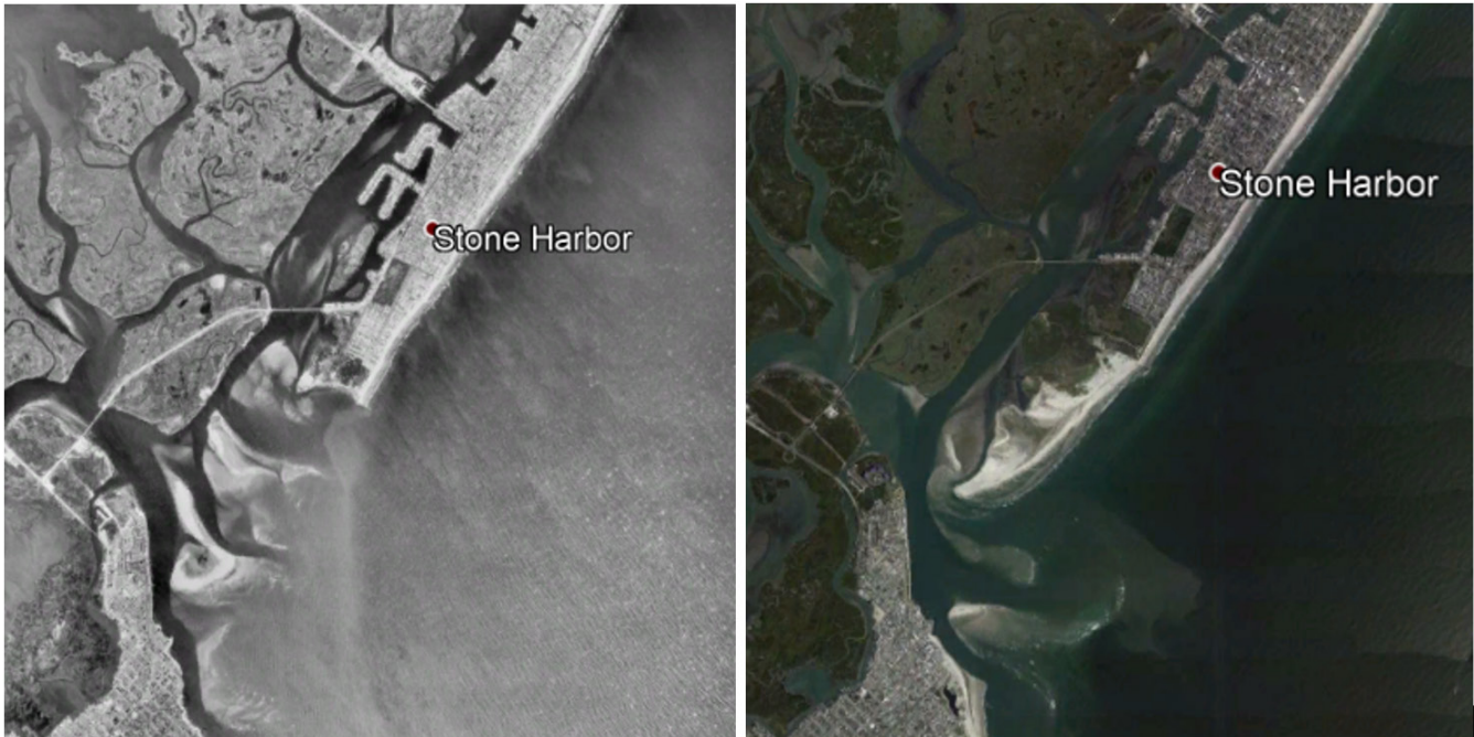
Stone Harbor Point [Left, Completely eroded (1994), Right, Fully restored (2016)] Image: Google Earth
