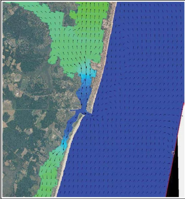
Figure 10. Model results showing velocity vectors of the tidal flux.
