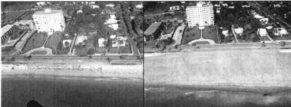
Figure 37 (above). Delray Beach before and after beach nourishment in 1973 (courtesy of Coastal Planning and Engineering, Inc.).
